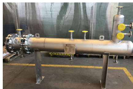
Titanium LL/H coalescer for water separation from acid solution.
