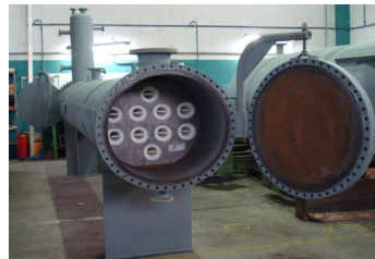
LL/H coalescer filter with integrated prefiltration stage for oily water.
