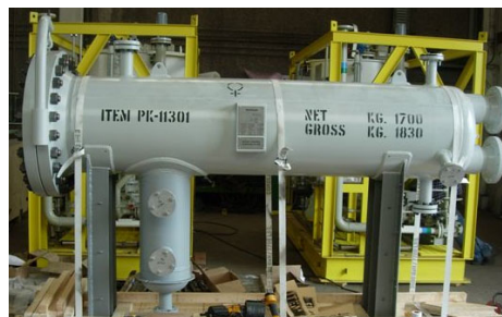
LL/H coalescer for caustic water separation from LPG.
