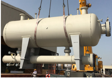
LL/H coalescer filter for water removal from ULSD (Ultra Low Sulphur Diesel).
